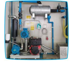
The diesel engine version allows the farmer to milk in the paddock and bypass the cost-intense job to get the animals back to the barn.
